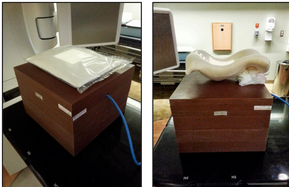
Figure 2 – Transmission measurement setup for new (left) and molded (right) headrest.
