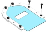
3. Insert the sleeves (if necessary) into the holes on the upper and lower frames. The sleeves should always be firmly pressed into the frames before inserting pins.
