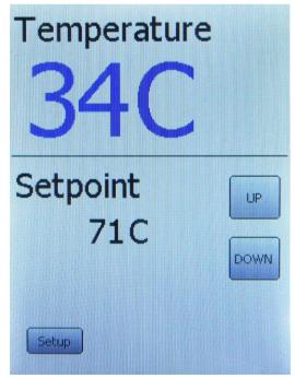
Buttons can be activated by a finger or medium soft object. Do not use knife or sharp pointed objects.
